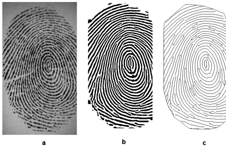
Fig. 6. (a) Original fingerprint; (b) an enhanced image of fingerprints; (c) the skeleton of fingerprints composed by a set of principal curves and the minutiae.
