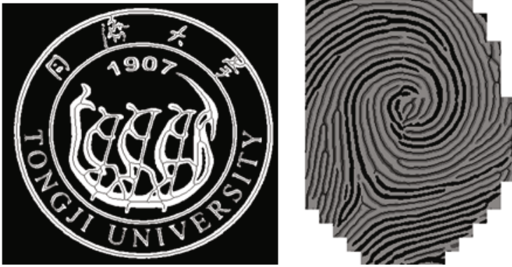
Fig. 3. Result of logo and fingerprint image skeletonization
