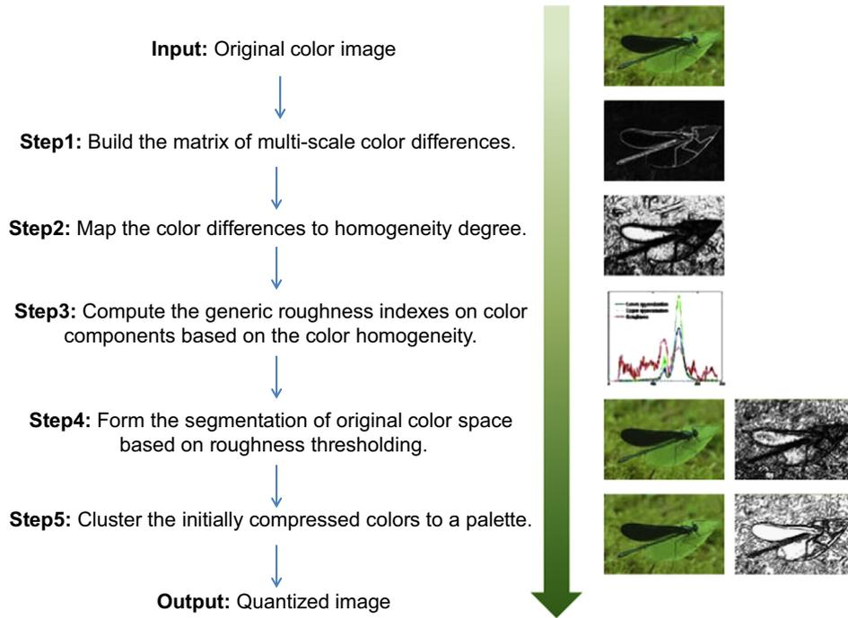
Fig. 2. The workflow of the quantization based on generic roughness measure.
