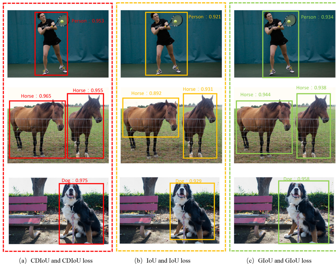
Fig. 11. Comparison of CDIoU-CDIoU loss, IoU-IoU loss and GIoU-GIoU loss under ATSS (backbone: _R_50_FPN_1x ) on COCO. CDIoU-CDIoU loss have better performance than IoU-IoU loss and GIoU-GIoU loss.
