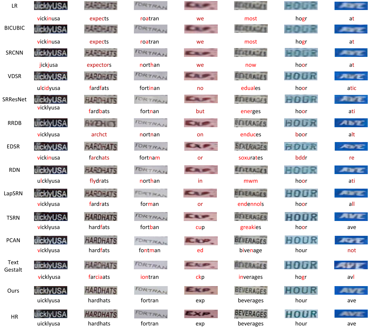
Fig. 8. Some visualization results of existing text SR methods on TextZoom [13] dataset, where the recognition results are provided by ASTER [4].
