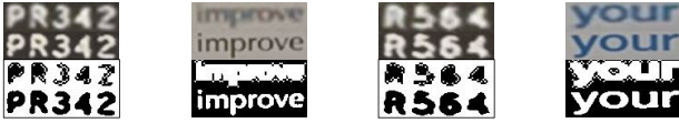
Fig. 2. Masks generated by calculating the average gray scale don't have a unified division of the stroke regions and the background regions.
