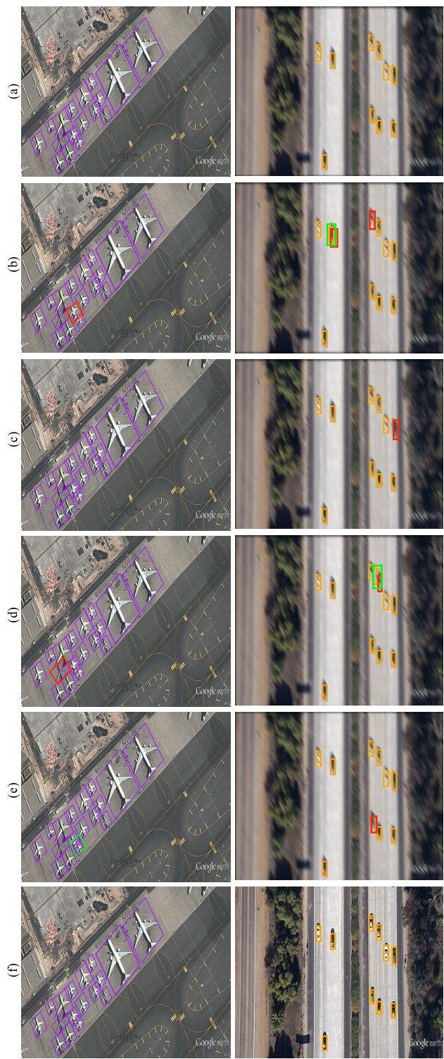
Fig. 12. Comparison of detection visualization results of different methods on UCAS-AOD. Each row represents the detection results of (a) ground truth, (b) DEA-Net, (c) Oriented RepPoint, (d) GF-CSL, (e) S 2 A-Net, and (f) proposed 3WM-AugNet. Green and purple boxes represent detected cars and planes, respectively. Red and green boxes indicate missed and false detections, respectively.
